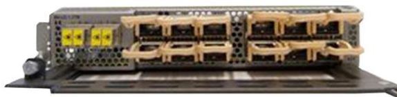
Figure 2. Cisco NCS 1004 1.2Tbps Line Card
